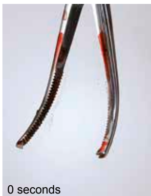
Photos: Arterial clamps with blood residue Sonication in the SONOREX SUPER RK 1028 ultrasonic bath with STAMMOPUR DR 8.
