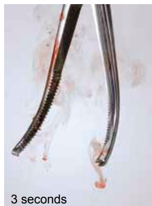
Photos: Arterial clamps with blood residue Sonication in the SONOREX SUPER RK 1028 ultrasonic bath with STAMMOPUR DR 8.
