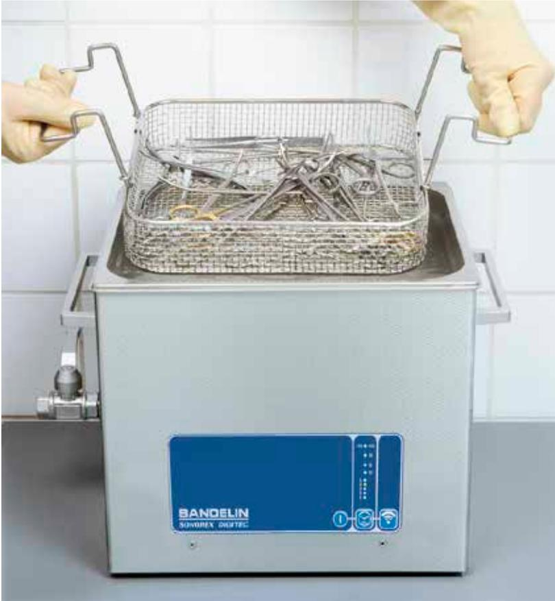
Instrument disinfection and cleaning in the SONOREX DIGITEC DT 514 ultrasonic bath.
