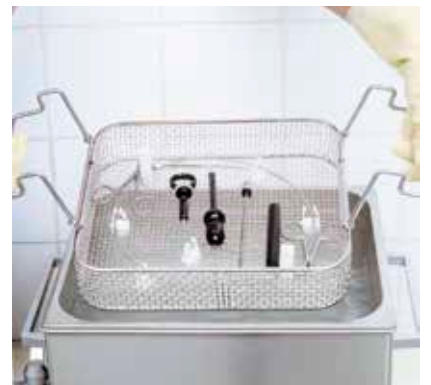
Disinfection and cleaning of endoscope accessories with fixing clamps FE 12. Practically affixed in insert basket K 14.
